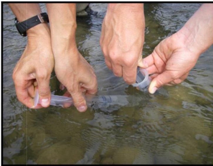
Figure 3.3. Application of a syringe periphyton sampler in the field.
