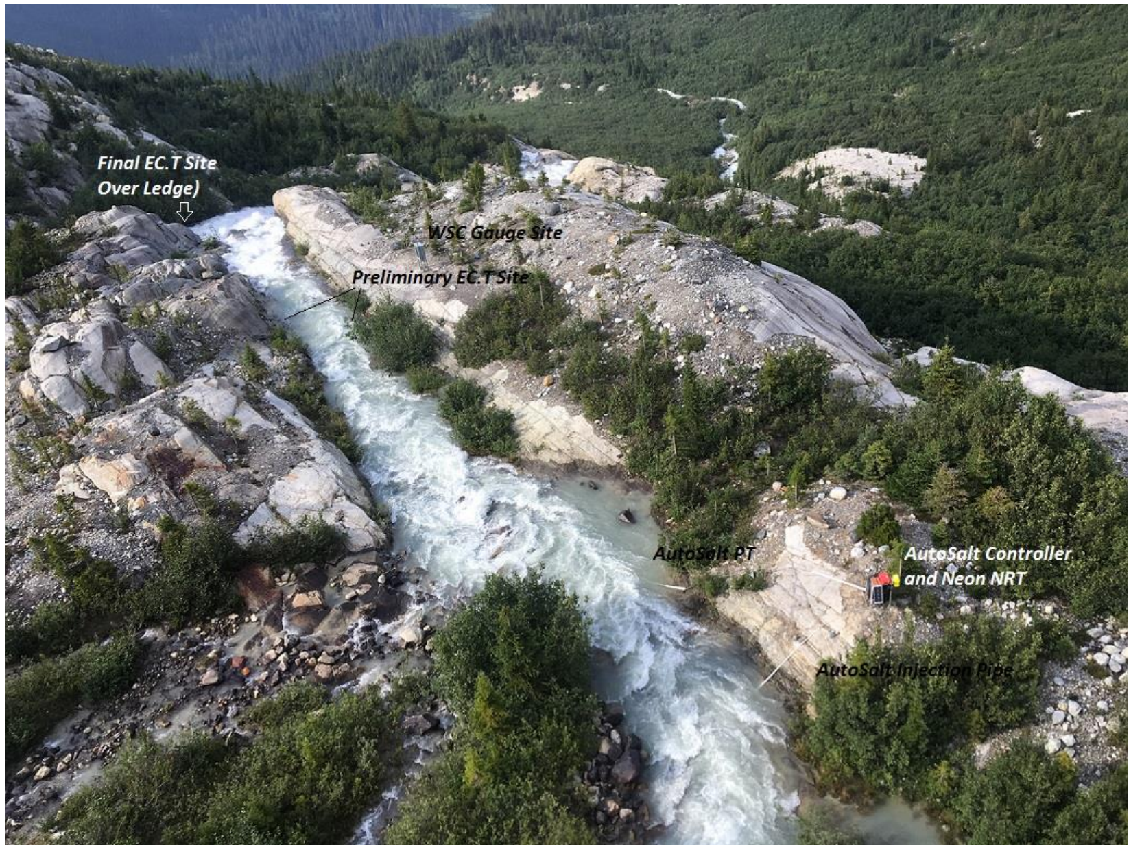
Installation of an automated salt dilution system Nordic Creek at outlet of Nordic Glacier (08NB020), Selkirk Mountains, BC
