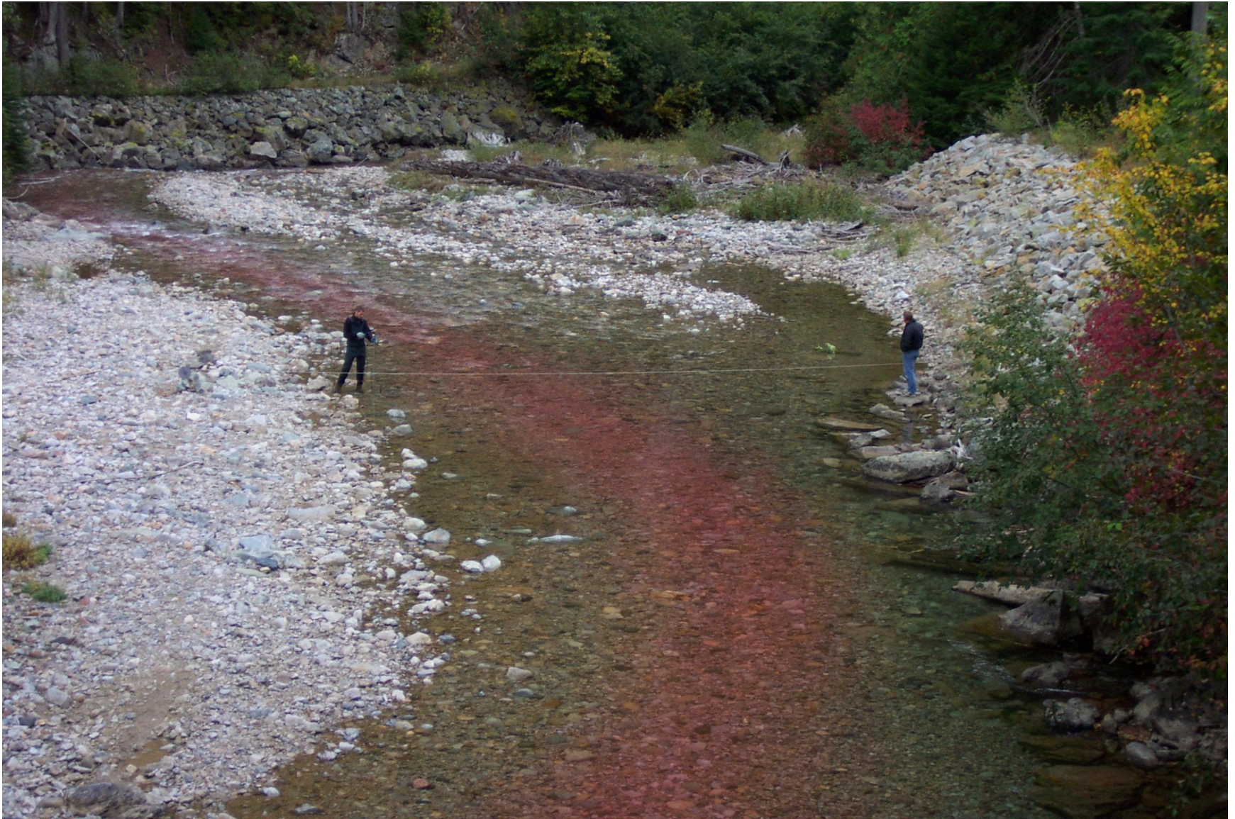
Example of poor lateral mixing of Rhodamine WT – Coquihalla River below Needle Creek (08MF062)
