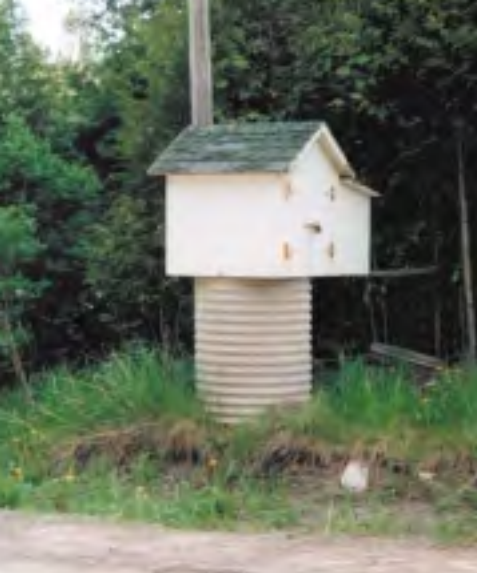
A stream gauge records water flows and levels
