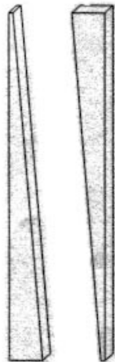
SAW 2 x 4 TIMBER DIAGONALLY TO PRODUCE 2 DEAD STOUT STAKES
