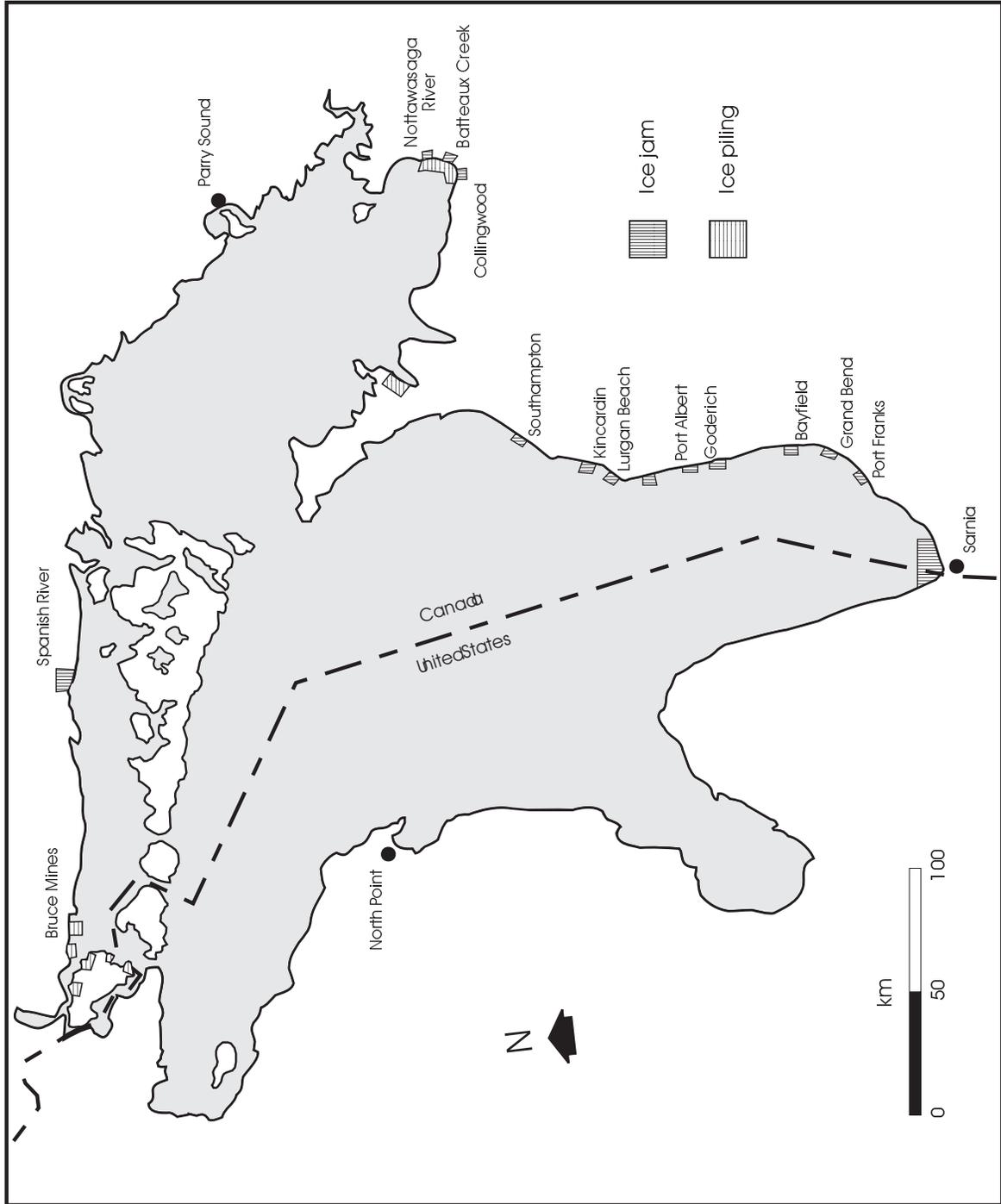
Figure A3.6.5: Ice and Ship Wave Flood and Erosion Prone Areas:
