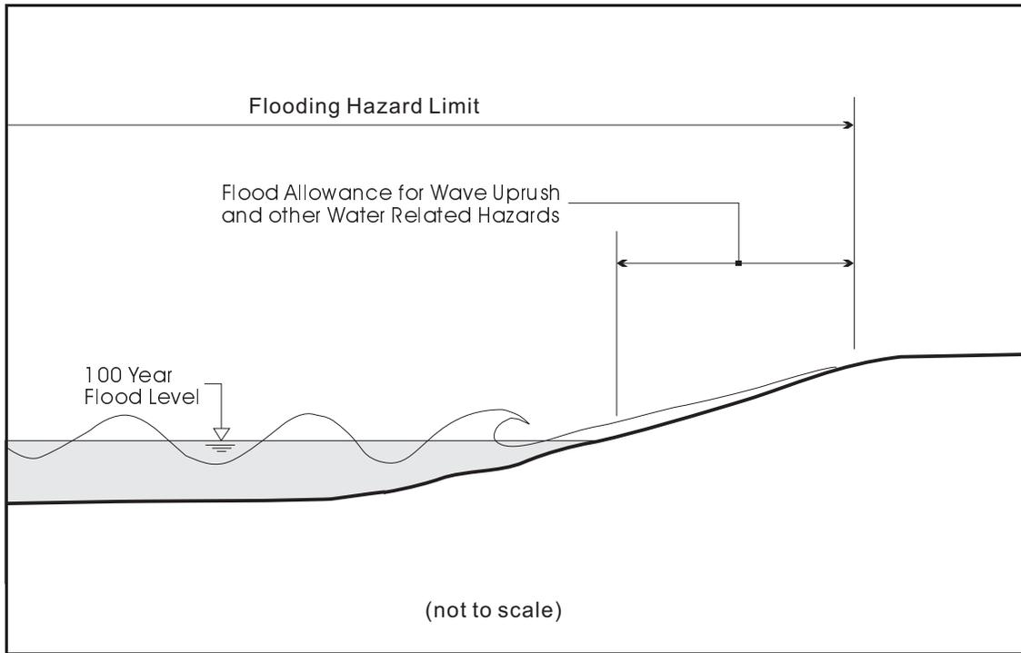
**Figure 3.5: Flooding Hazard Limit - Standard 15m Flood Allowance for Great Lakes**
