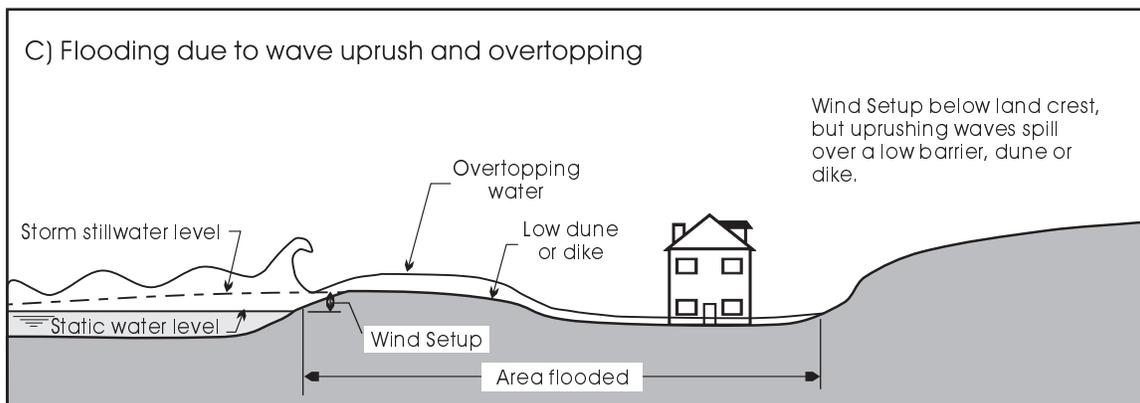
Figure 3.3: Wave Uprush and Wave Overtopping
