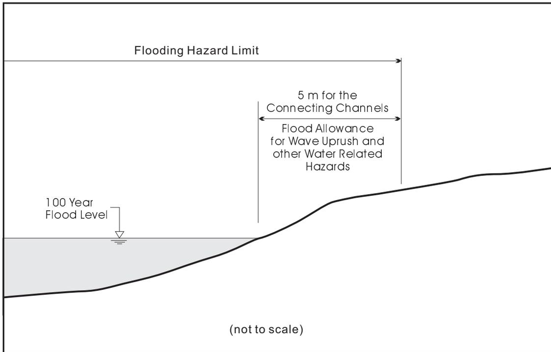
**Figure 3.7: Flooding Hazard Limit with Overtopping**
