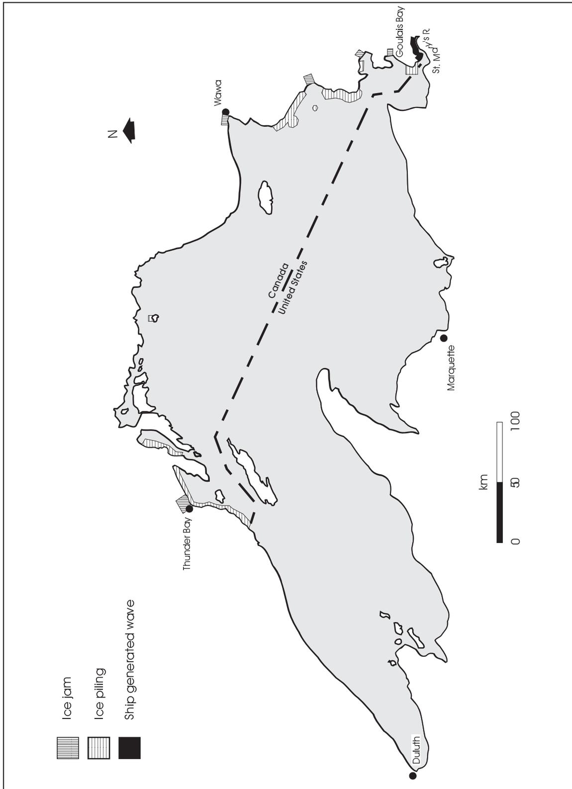
Figure A3.6.4: Ice and Ship Wave Flood and Erosion Prone Areas: Lake Huron
